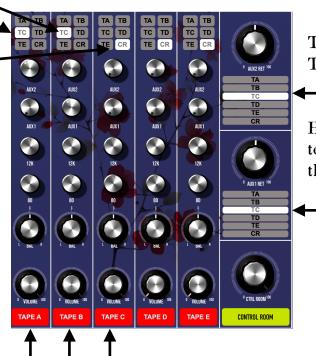
TAPE A and B are routed to TC TAPE C is routed to CR
