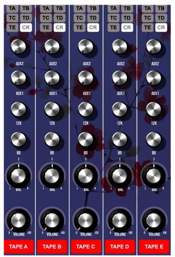
The Tape Return Channels A,B,C,D,E have a simple EQ (LOW-HIGH) and 2 AUX Sends. Aux 1 is routed to the DELAY, Aux 2 to the REVERB. The DELAY and REVERB Returns can be routed to the tapes in case you want to record the efxs.
