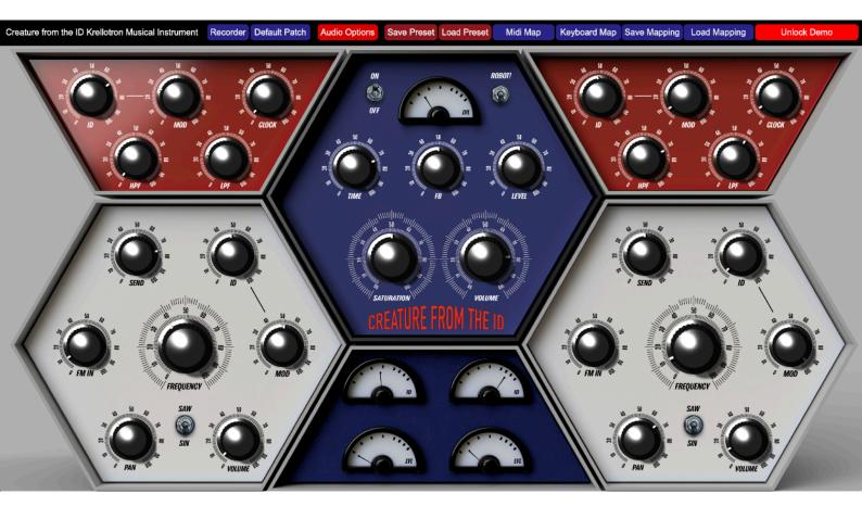
CFTI has 2 identical sound generators and a master interface at the center, with delay, saturation and output volume control. The sound can be recorded in a separate window: see RECORDER.
