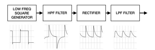
Let's say we have a 2Hz square waveform, if we apply a first order High Pass filter (Cutoff equal or > 2Hz) we get a sort of exponential fall at the end of the cycle. We then rectify the waveform so we obtain a simple AR curve with exponential release. An LPF filter can be used just after that to smooth the attack. The signal is then sent to a ring modulator to control the amplitude of the generator's sound.
