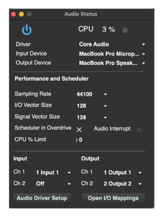
The blue I/O button at the left turns on and off the audio scheduler. If you modify some settings you must to restart the audio processing by turning off and on again this blue button. If it is yellow it means that you need to restart the audio scheduler.
